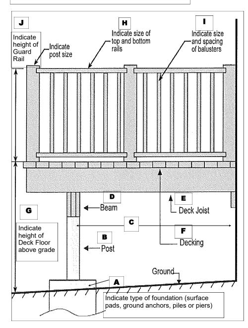
All structural elements must be attached with appropriate fasteners. <u>Deck screws are NOT structural.</u>
